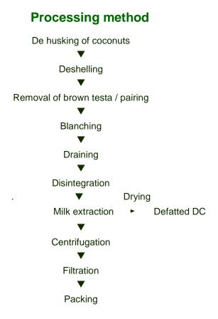
**Dehusking**: Husk is removed manually or with the help of coconut dehusking machine. **Deshelling**: It is done to remove the shell of the coconut. This is done without breaking the
